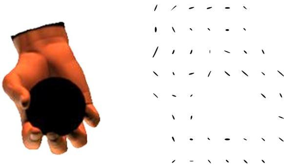
Fig. 3. The left image shows an example from the database. The right image shows the associated image feature descriptor  $y$ . Prior to extracting the feature descriptor the object is segmented from the image, resulting in a “hole” at the corresponding position in the descriptor. This encodes the correlation between pose and object in a more robust manner compared to if the internal edges of the object would also contribute to the descriptor.
