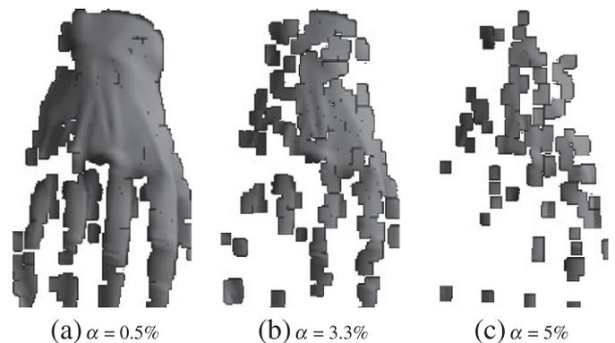
**Fig. 7.** Artificial corruption of the segmentation of the synthetic test data. The corruption is performed as follows: A partial segmentation is created by randomly removing  $\alpha$  percentage of the pixels from the segmentation. The morphological operators of erosion and dilation then applied this partial segmentation in order to propagate the noise over the image. Examples of increasing segmentation noise are shown.
