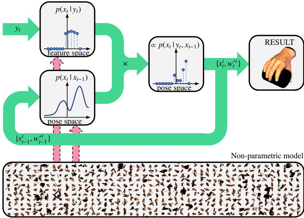
Fig. 2. Schematic figure of the non-parametric temporal pose estimation framework. Given an image observation  $y_t$ , a set of pose hypotheses  $X_t$  are drawn from the model. Each hypothesis is given a temporal likelihood based on consistency with the hypothesis in the previous frame. The final estimate is the pose associated with the largest probability.
