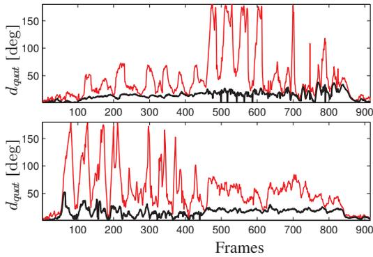
Figure 9: Error curves for video-based tracking (red) and hybrid tracking (black) obtained for an arm rotation sequence (first performed by the right and then by the left arm). **Top:** Left hand. **Bottom:** Right hand.
