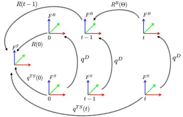
Figure 6: Integration of orientation data into the video-based tracker. *Ground-truth orientation*: clockwise down path from  $F^S$  at time  $t$  to  $F^T$ . *Tracking orientation*: anti-clockwise upper path from  $F^S$  at time  $t$  to  $F^T$ .
